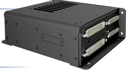
The JACS-001 Audio Control System is designed to distribute and control all the transceiver, receiver, aural messages, microphone and intercom audio within the aircraft. Multiple users may operate the system via a choice of control panel types that communicate with the JACS-001 to set audio controls and relay system information.
