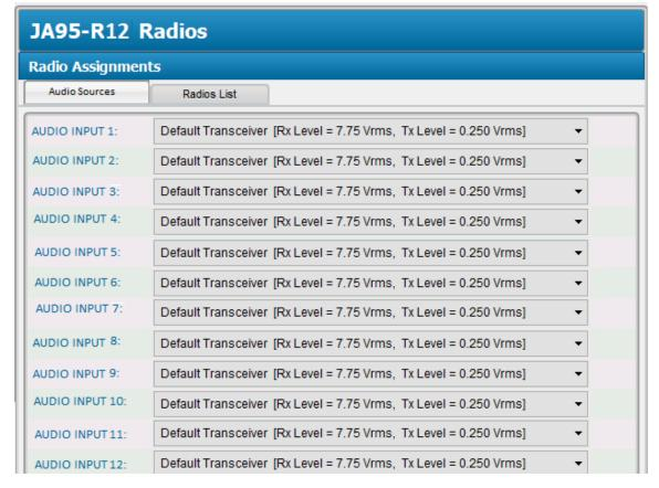
The Radios window is used to define the radios for the audio sources.
