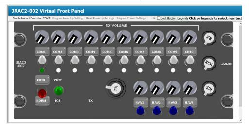
This Virtual Control Panel is used to define the 'names' associated with the control legends. The selected name will be used in all subsequent references to the associated transceiver/receiver, and will be used on the custom-generated Connector Maps and Interconnects.
