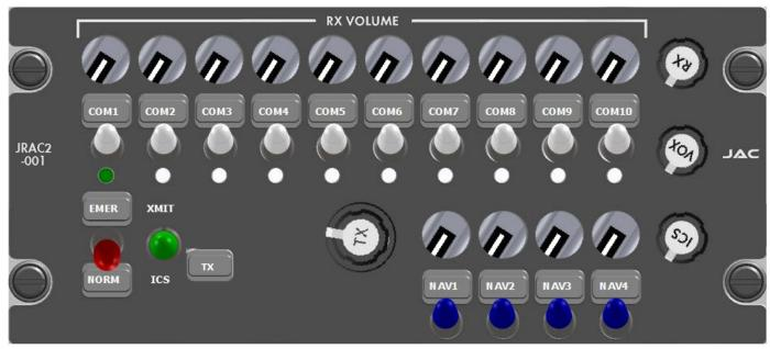
From the Virtual Control Panel the operator may use the mouse pointer to change the position of the virtual switches and rotary controls; and observe the status of the Transmit Select Annunciators and the Transmit Annunciator.
