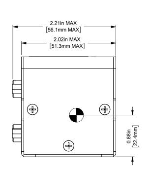
$\bigoplus_{\pm 0.03 \text{in } [0.8 \text{mm}]} \text{CENTER OF GRAVITY}$
