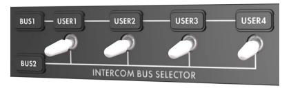
If it is a requirement for **ALL USERS** to be able to talk together on the intercom, all users' switches must either select BUS 1 or BUS 2 (i.e. all switches in the same direction.)
